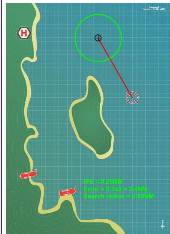
2) A boat has contacted the coastguard stating that it has run out of fuel. They've given their coordinates from their onboard GPS shown on the map. This report has an IPE (initial position error) of 0.25 NM (nautical mile).
